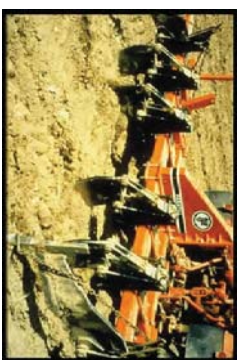
Fig. 13. The same deep, angled-leg subsoiler shown in Fig. 7 is engaged at maximum depth for Phase 2, decompaction (deep soiling), of the replaced topsoil and the upper subsoil materials.
