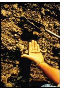
Fig. 5. Augered from a depth of 19 inches below the surface of the replicated topsoil, this subsoil sample was hand rolled to a 1/8-inch diameter. The test shows the soil at this site stretches out too far without crumbling; it indicates the material is in a plastic state of consistence, too wet for final decompaction (deep subsoiling) at this time.
